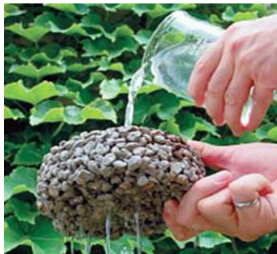
FIGURE 3-5 – Example of function of permeable pavement
