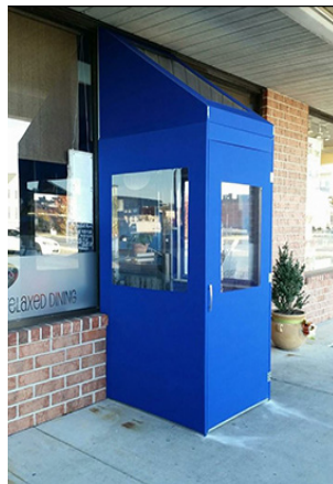
Figure 14: Installing a sidewalk vestibule enclosure can prevent winter draft and help control indoor temperature to improve building occupants' thermal comfort. (Source: New York City Signs )
