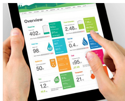
Figure 21: Energy Management System can be accessed online and provides real-time energy use monitoring which can indicate any energy inefficiencies in the building. (Source: GPSIntegrated )
