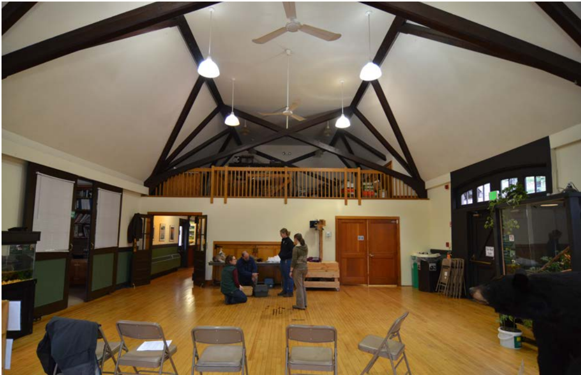
Figure 16: Ceiling lighting in the Nature Center's largest education space is controlled by one on/off switch.
