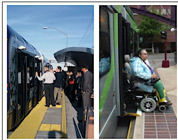
Figure 22: Level (Las Vegas MAX) and near-level boarding (EmX) platforms facilitate accessibility. Note that near-level requires a ramp and therefore a longer stop. Source: APTA
