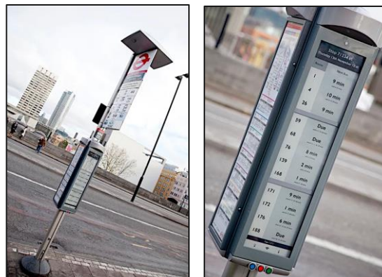
Figure 32: Screens in London, use e-ink to present information, and 3G to send scheduling and map data. Source: New Atlas 266
