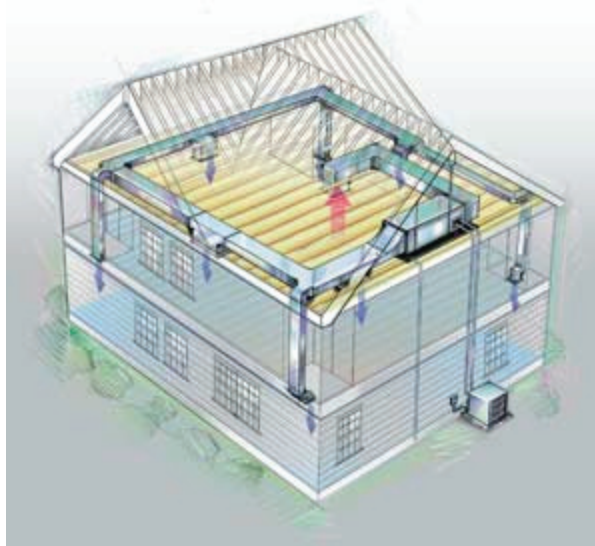
Figure 32 - Overview of how central air is incorporated into a house 103
